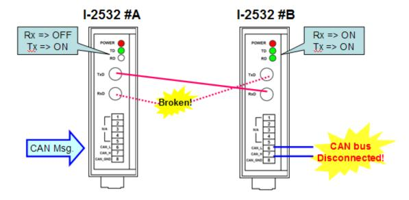
(4) One channel (Tx side) of the fiber cable is broken.
