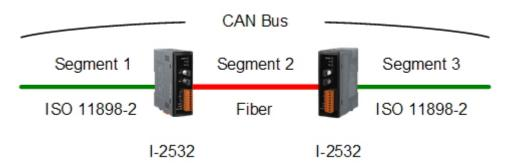
If some bus error, except the short of the CAN\_H and CAN\_L, happens in the Segment 1, the CAN error message will be transferred to the Segment 3 and vice verse. The short of the CAN\_H and CAN\_L have no affection to another Segment. That is, the CAN data exchange in the Segment 1 works normally even if the CAN\_H and CAN\_L are shorten in the Segment 3. The CAN message transformation between Segment 1 and Segment 3 is terminated while the Segment 2 is broken. (2011/1/5,Bear)
