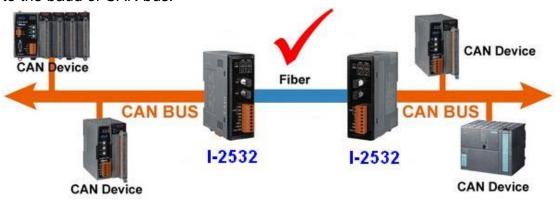
2. Use a couple of I-2533s. The working distance of fiber is fixed. The maximum length is 2 km.
