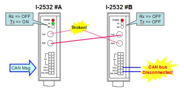
(5) Different CAN baud rate on the two I-2532 modules.
